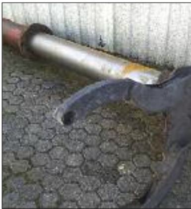
removed old piston with lifting head
